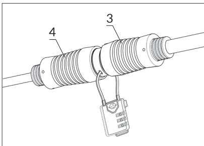
Pass the cable through the holes in the adapter and plug and lock the padlock with the TSA (Travel Sentry Approved) system, with a triple cipher combination. The use of such a padlock does not require carrying a key, which can be easily lost.
