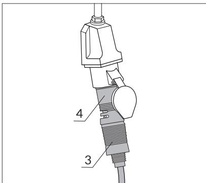
► To lock the connector press the plug and adapter together.
