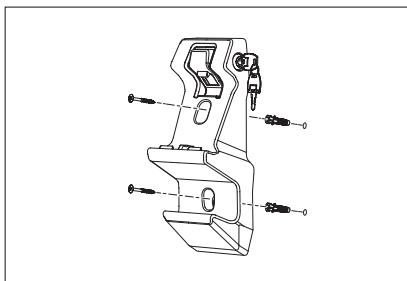
To protect the device from theft, the hanger can be locked with a key (1).
